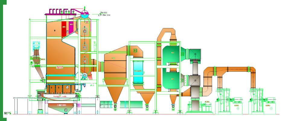
TYPE: Bi-Drum Bottom Supported,<br/>IndoorCAPACITY: 60 TPHFUEL: Palm Fibre / EFB: 31 bar(g)FIRING SYSTEM: Spreader, Traveling grate° CSOOT BLOWERS: LRSB/RSBTHERMODYNE
